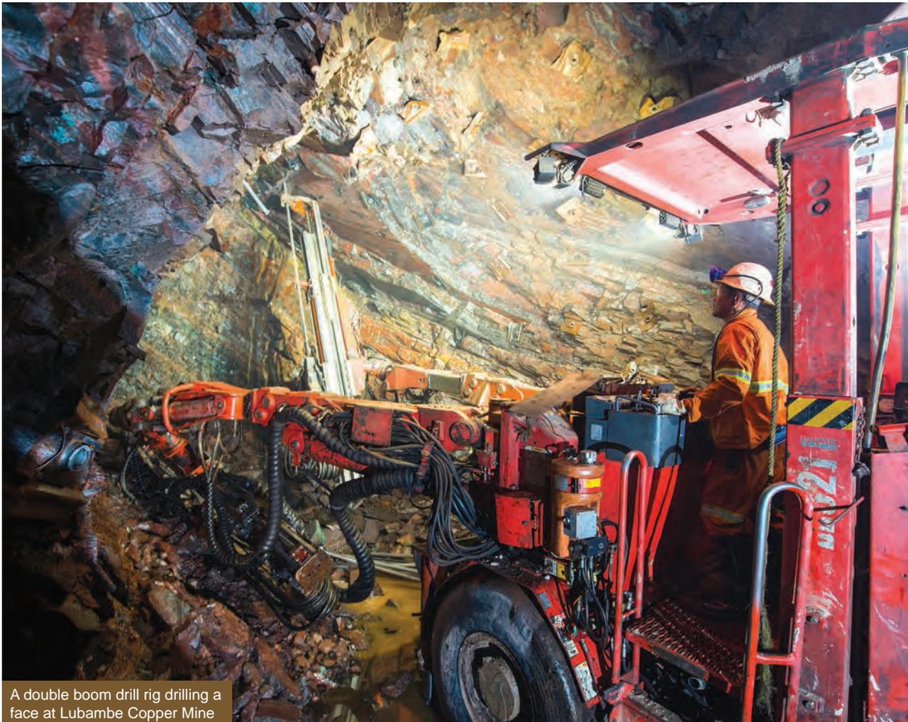
A double boom drill rig drilling a face at Lubambe Copper Mine
